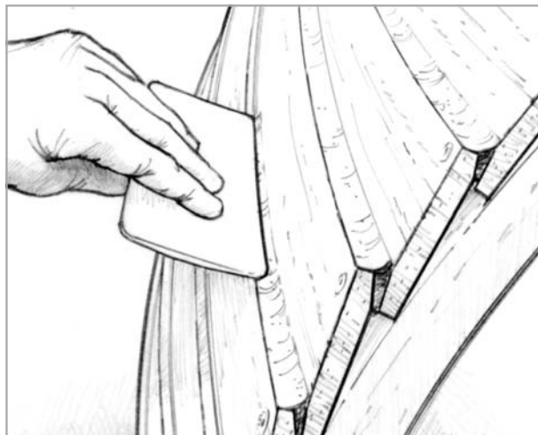
Figure 5-9 Fill the wet-out seam with thickened epoxy
