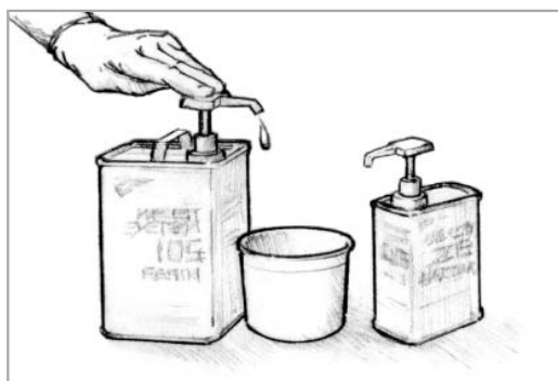
Figure 8-4 Dispense the proper proportions of resin and hardener.
